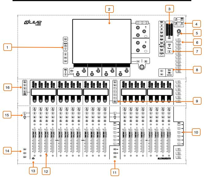
**Channel Processing** – Press a fader strip **Sel** key to access the processing for the input or mix channel assigned to it. Read the Harmony UI paragraph below for further information.
