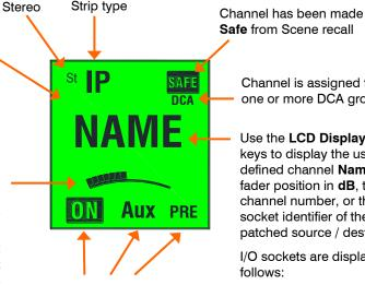
Assignment to the active Mix, Mix type and pre/post setting
