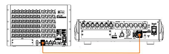
Switch on the Surface. The gigaACE Lnk/Err indicators flash at a steady rate when the link is established. The red error indicator lights if a communication error is detected. Check that the cables are correctly plugged in and are not faulty.
